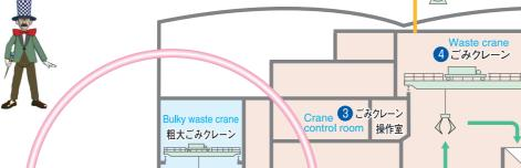
**Waste Dumping** Waste is dumped into a pit 2 through waste pit doors 1. It is then dropped by a crane 4 which is operated remotely from the crane control room 3, into a feeding hopper 5.
